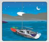
The masthead light and sternlight may be combined as an all-round white light on vessels less than 39.4 feet long.
