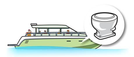
Boats operating on state waters with an installed toilet must also have a sanitation system to prevent pollution and discharge of raw sewage. A typical sanitation system consists of: an installed toilet, a waste treatment system, or MSD, and/or a holding tank.
