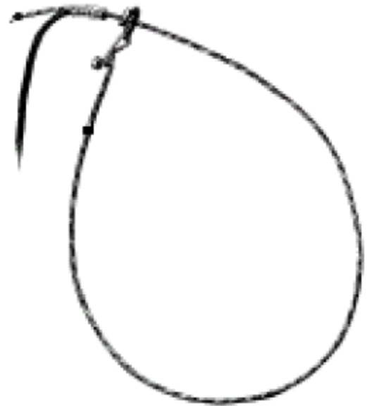
An improperly loaded cable loop appears as a tear drop shape. Resistance in the cable loop makes it difficult to fire properly.
