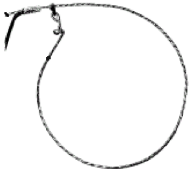
A properly loaded cable loop is shaped more like an oval or kidney.
